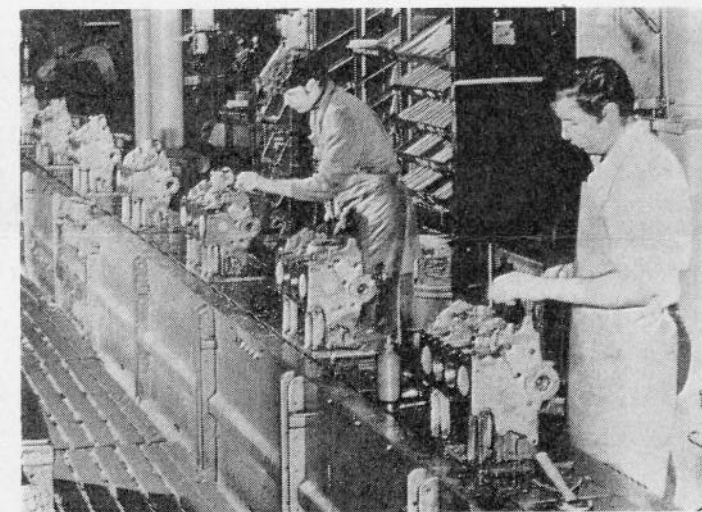
Part of the assembly track for reconditioning engines. Over 60,000 engines are processed every year
