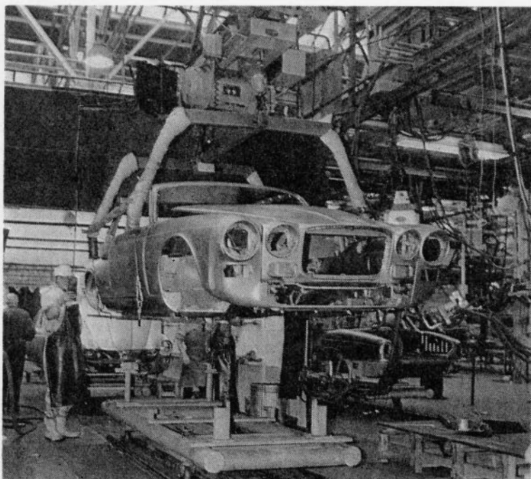
The Jaguar XJ6 body shell is completed at the Castle Bromwich Birmingham works of Pressed Steel Fisher.
