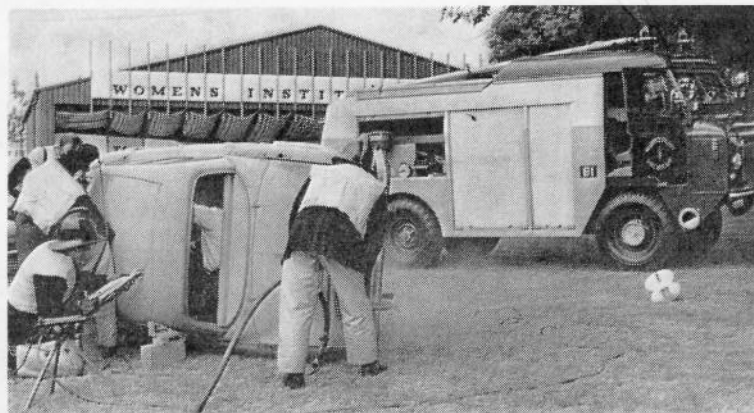
Members of the Warwick County Fire Brigade with their specially-equipped Forward Control Land-Rover, demonstrate the facilities offered by the vehicle for tackling accidents on the motorways. Special discs and cutting equipment are available for rescuing trapped passengers in damaged vehicles.
