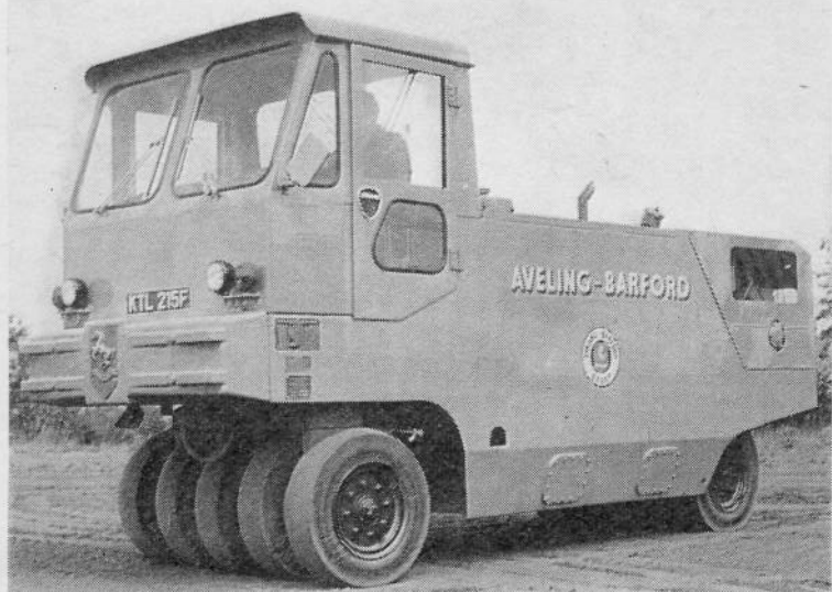
The nine wheeled pneumatic-tyred roller. Wheels are mounted in pairs, the rear four covering the gaps between the front five.
