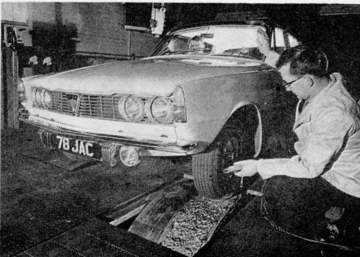
A Rover 2000 mounted on a roller track fitted with special segments for sound vibration tests in the Dunlop Chassis Laboratory.
