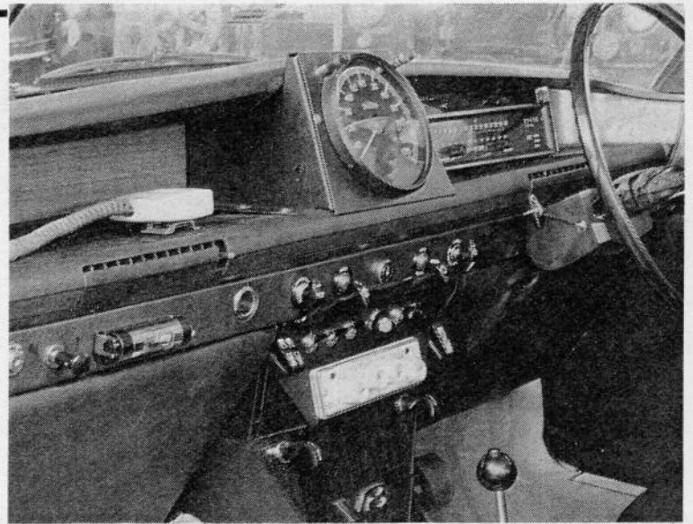
Note the large fully calibrated speedometer and radio telephone.
