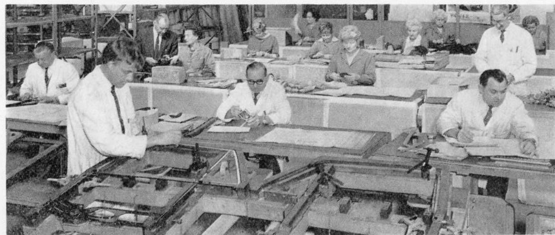
Inspectors at work on bought out materials on stage three of Rover 2000 assembly. The man in the foreground is checking a door frame.
