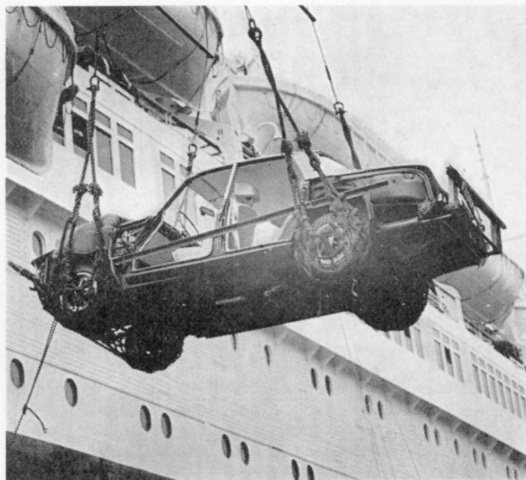
Gripped firmly in a rope net, the Rover 2000 TC is hoisted up the side of the Queen Mary to the platform from which the car was manhandled into the liner. Body panels and doors have been removed for the operation.
