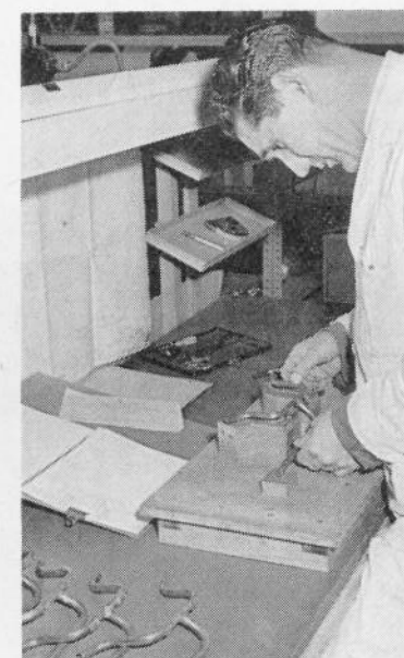
Mr. G. Hughes (Receiving Inspector, Solihull) tests a bought out item on a fixture, with the drawing, inspection and record cards on hand for reference.
