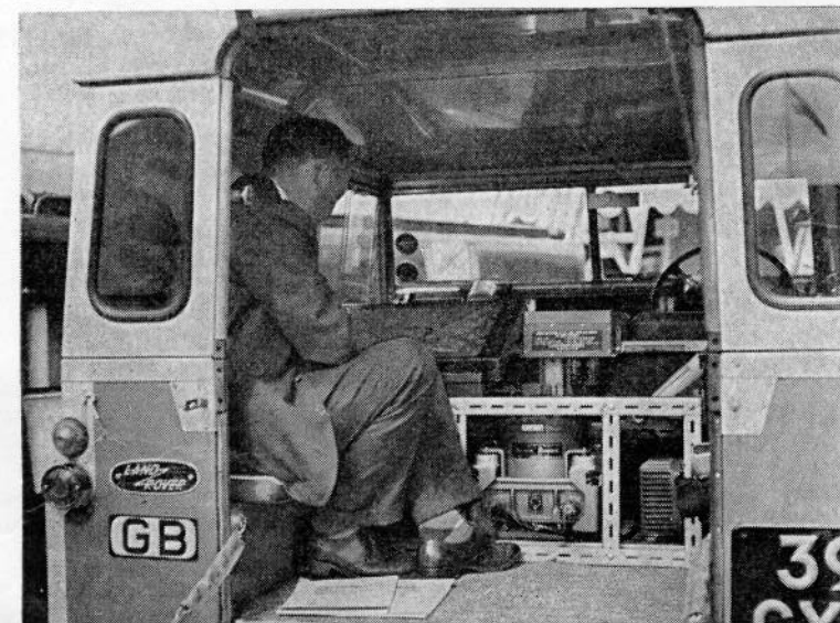
An operator demonstrates the gyro-controlled navigation system installed in a Land-Rover and exhibited at Farnborough.
