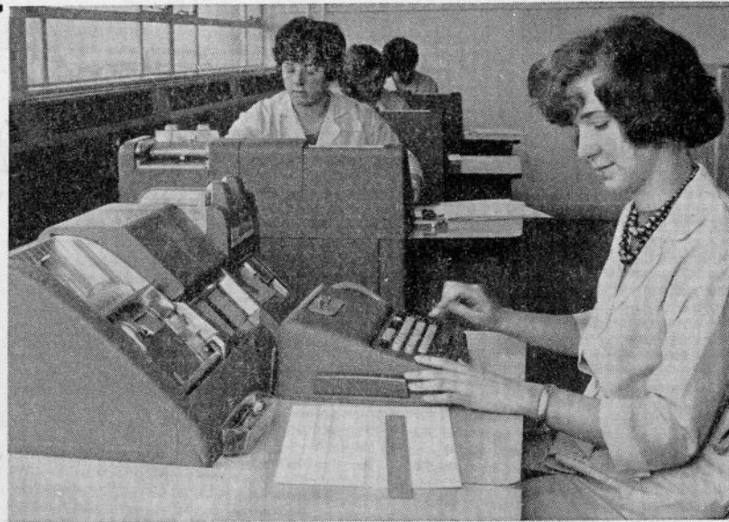
LEFT: The computer block at Solihull as seen by passers-by. ABOVE: Information for the computer being punched into cards by girls in the preparation room. This operation is also carried out in Hollerith. From foreground to the rear of the room are Miss Ann Goodyear, Miss Helen Rose, Miss Janet Dutton and Miss Janet Grindrod.
