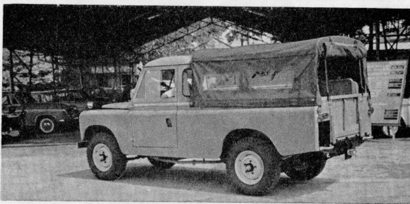
Remember seeing the above picture in last month's issue of ROVER NEWS? It was of a Long wheelbase Land-Rover after being extensively damaged by a mine in Vietnam. As can be seen from the photograph below, the vehicle proved to be indestructible and was as good as new after repairs by Societe Indochinoise de Transports, of Saigon, our Vietnam distributors. Only certain parts of the chassis and body had to be changed on the vehicle which, before the mine incident, had already done 80,000 kilos.
