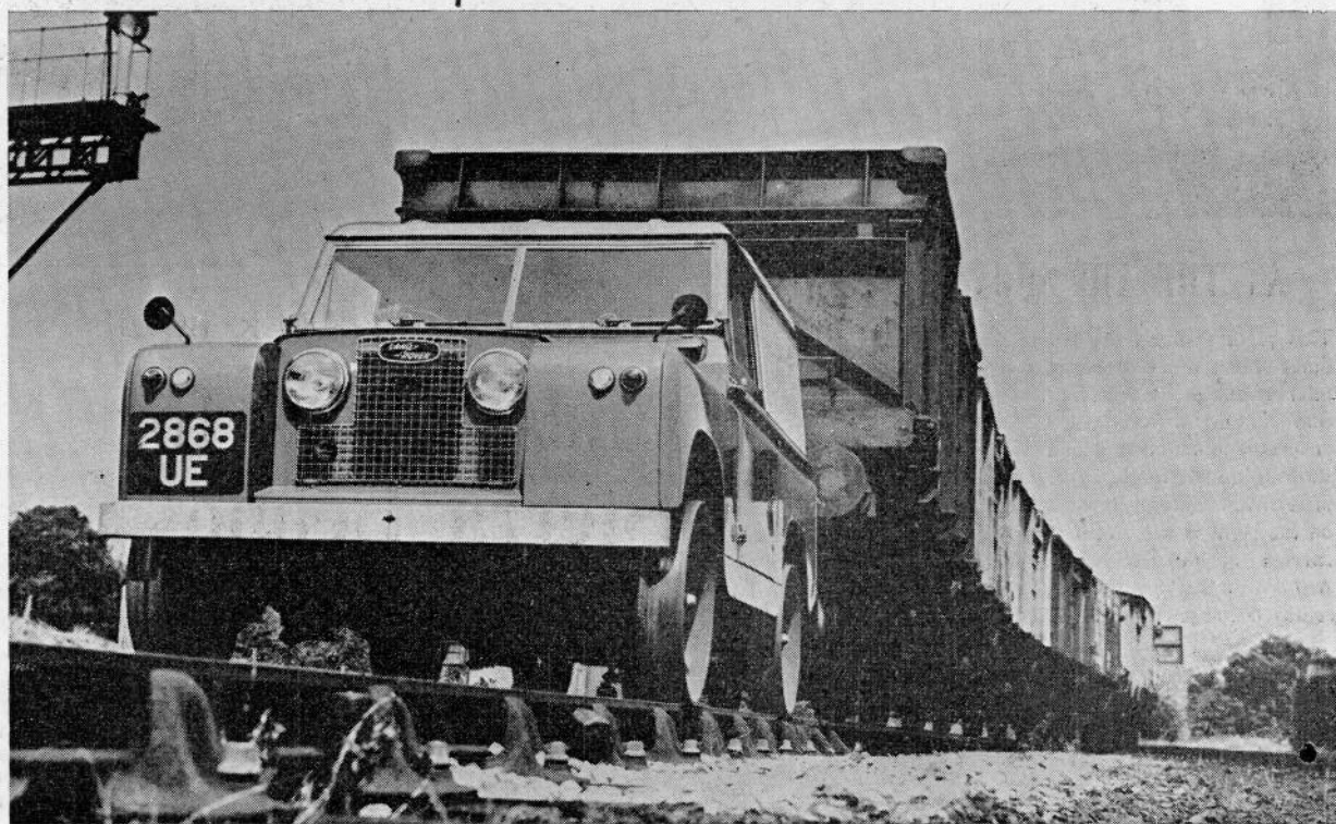
A striking illustration by a "road-railer" conversion of the new Diesel Land-Rover's pulling power.
