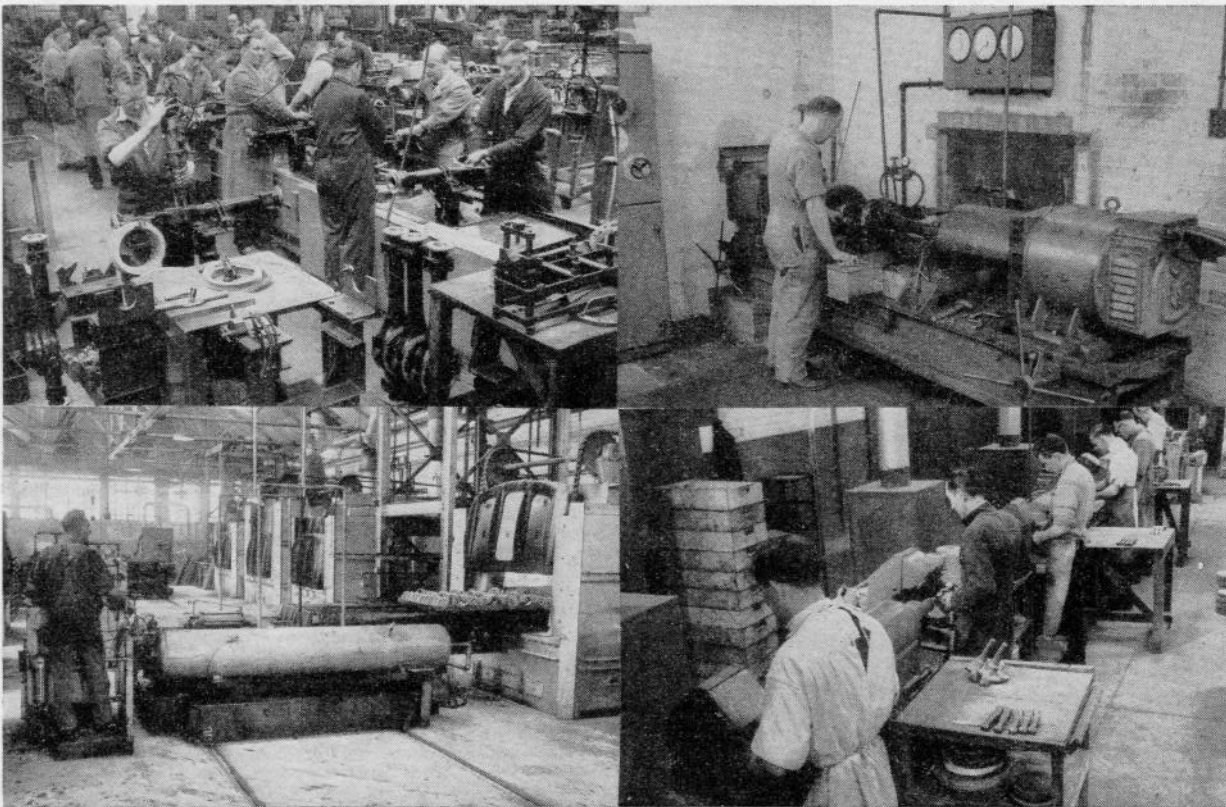
Inside Perry Barr factory . . . the front axle assembly track makes a busy scene (top left) while Mr. F. Walker is seen (bottom left) handling the charging unit for the hardening furnaces. A section of the Polishing Shop is seen in the bottom right-hand picture, and the fourth picture shows Mr. D. Adam operating a rear axle testing unit.
